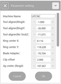
Interface 3: tool configuration button. The tool library information of the current device is shown under this tab. The tool positions of the current tool library can be adjusted or filled in, and saved by clicking the tick button.
