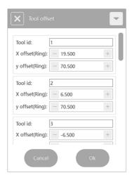
(3) Parameter configuration interface: check the calibration ring coordinates
