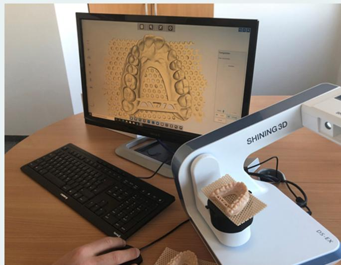
In order to determine deviations in production in the 3D printing process from the original data (CAD files), to visualize them and to be able to analyze them quickly and precisely, a target-actual comparison is created. This also serves to minimize position and shape tolerances in the production process and to optimize the 3D printing process with regards to correct print settings.
