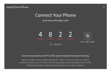
Transfer **Raw** data from a phone to a PC. Ensure the phone and PC are connected to the same Wi-Fi network. Do not minimize the app or turn off the phone's display screen during the file transfer, or the transfer will fail.
