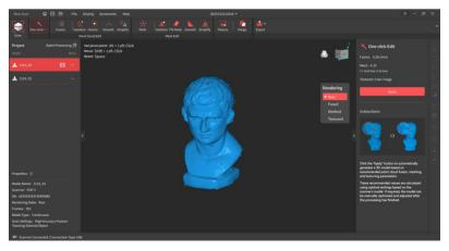
After scanning, process the scan as required. Revo Scan provides a **One-click Edit** function for new users and allows experienced users to perform Fusion, Mesh, and Texture step by step.
